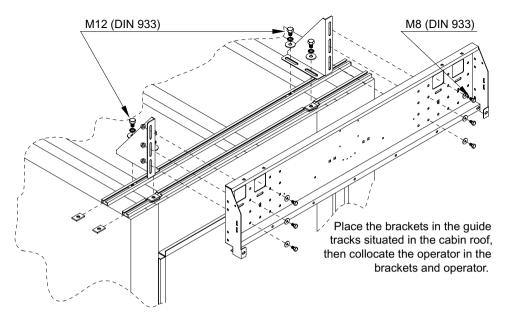
By means of the slits in brackets and the existing holes in the operator, regulate the height up to 2220 mm in the operator extremes. Leave a distance of 30 mm
